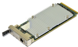
AMC-2C6678 2x6678+FPGA AMC card
